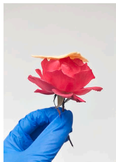
Fig. 4. Digital photograph of the \text{SiO}_2/\text{PI}/\text{AF} aerogel composite fabric laid on a flower.
